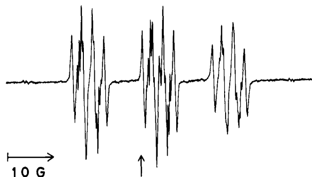
Figure 1. ESR spectrum of an aqueous solution of L-Ala-Gly with MNP observed just after \gamma irradiation (at pH 5.5). During chromatography the magnetic field was fixed at the position indicated by the vertical arrow.
